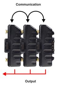
PAGlink also allows batteries to be hot-swapped for continuous power, which means no more time-wasting camera reboots while shooting. Intelligent PAGlink batteries form a network when linked, allowing them to communicate with each other and manage output safely and efficiently. The batteries do not discharge into one another.
