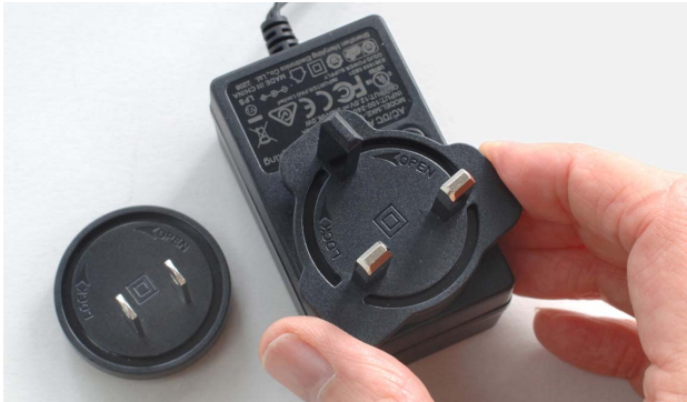
Fig. 1. Fit the appropriate plug to the Power Supply Unit. Align the plug and rotate it clockwise into position until it locks with an audible 'click'.
